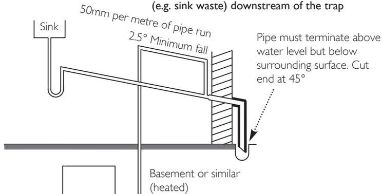
vi) pumped into an external soil & vent pipe
