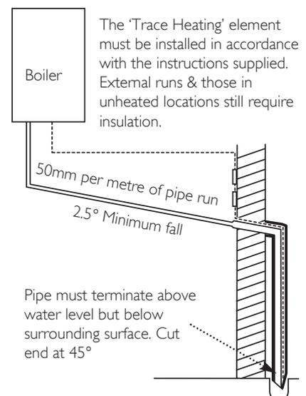
The 'Trace Heating' element must be installed in accordance with the instructions supplied. External runs & those in unheated locations still require insulation.
