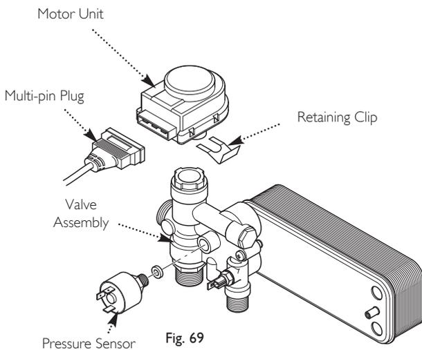
1. To replace the motor unit, disconnect the multi-pin plug.
