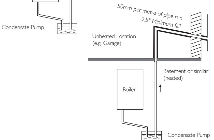
vii) to a drain or gully with extended external run & trace heating
