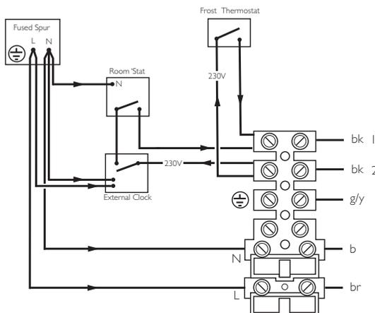
**NOTE:** The 230V switched signal for external controls (Frost Stat - Room Stat - Timer) must always be taken from terminal 2 at the boiler. Live, Neutral and Earth to power these controls must be taken from the Fused Spur.
