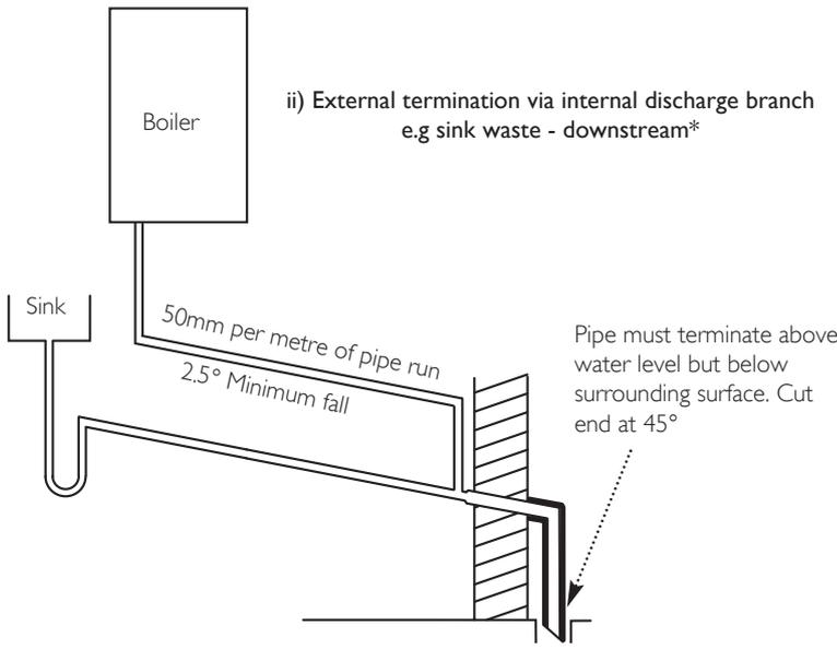
\*It is **NOT RECOMMENDED** to connect upstream of the sink or other waste water receptacle !
